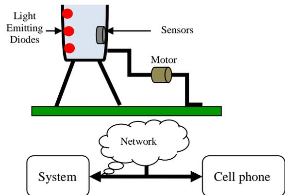
Fig. 1. Water Monitoring System [5]
