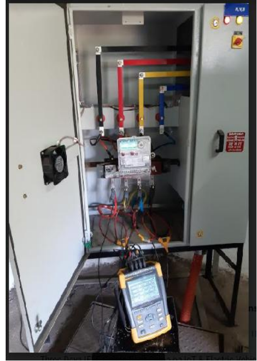
Fig. 4. Harmonic Measurements at site
