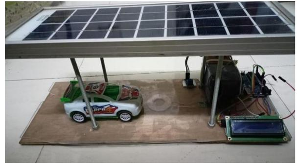
Stage-2: LCD displays the Solar voltage.
