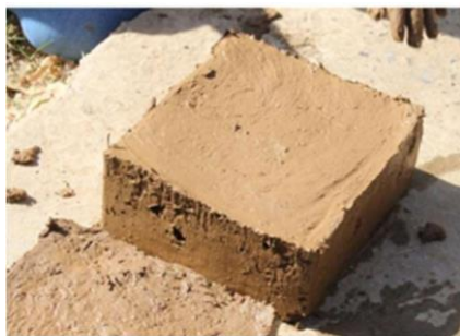
Fig 12 Wet Wardha Block for Interior walls
