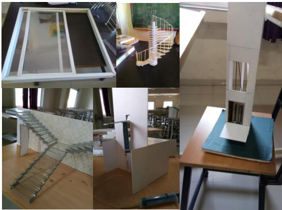
Fig.5) Working models by the students of D.Y. Patil School Of Architecture of Sliding window, Spiral staircase, Glass staircase, Hydraulic lift using Injection to apply the pressure.
