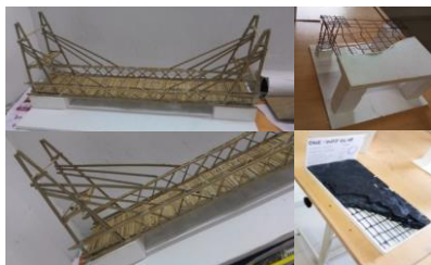
Fig.3) Models done by students of B.D. College of architecture to understand load transfer in long span bridges and one way two way slabs.
