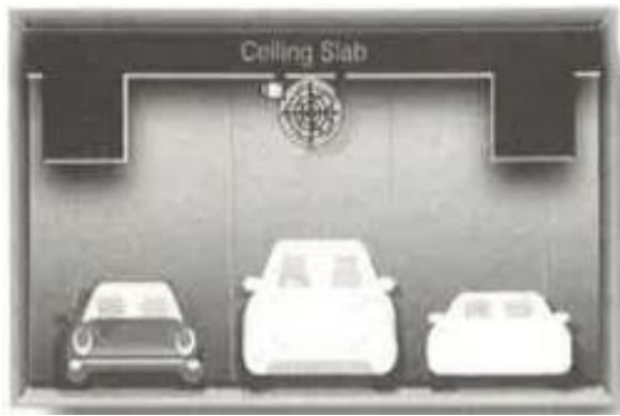
Fig: 5 placing of Ductless Ventilation
