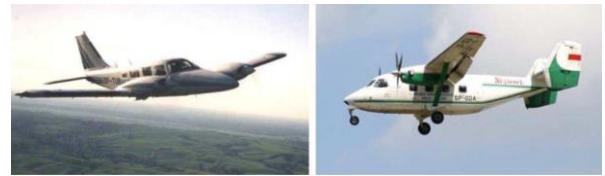
Fig. 6. The six-seat PZL M20 'Mewa' civilian airplane (on the left) is utilized as a flying testbed, whereas the PZL M28 'Skytruck' commuter aircraft is employed as a modeled reference.
